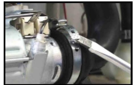
To release the hose clamps, it is recommended that this assembly be taken off its hinges.
