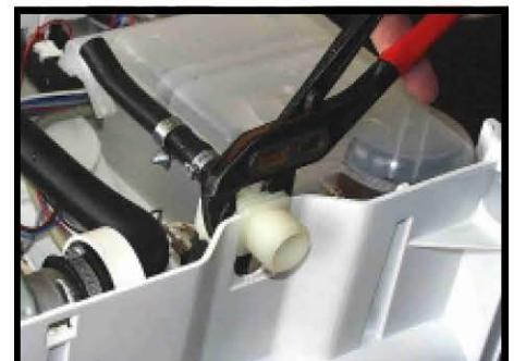
After the removal of the hose, the valve can be drawn out of the chassis with suitable pliers.
