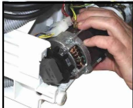
After loosening the screws of the two holders and the yoke, the circulation pump pump/continuous flow heater unit can be taken out.
