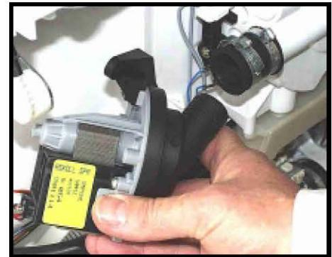
To dismount the leach pump, the hose clamps are released and the screws removed.
