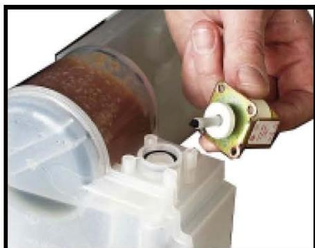
After undoing the screws of the recycling valve, this can be removed.
