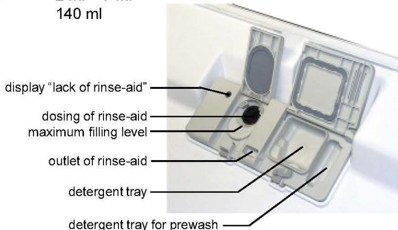
The detergent compartment 1 is filling corresponding to the set dosing quantity when the door is open. Possibly existing rinse-aid in compartments 2 and 3 flows back into the storage tank of the rinse-aid. The detergent trays are filled up. The door will be closed and the detergent for prewash will be rinsed out through the slots in the detergent dispenser cover.
