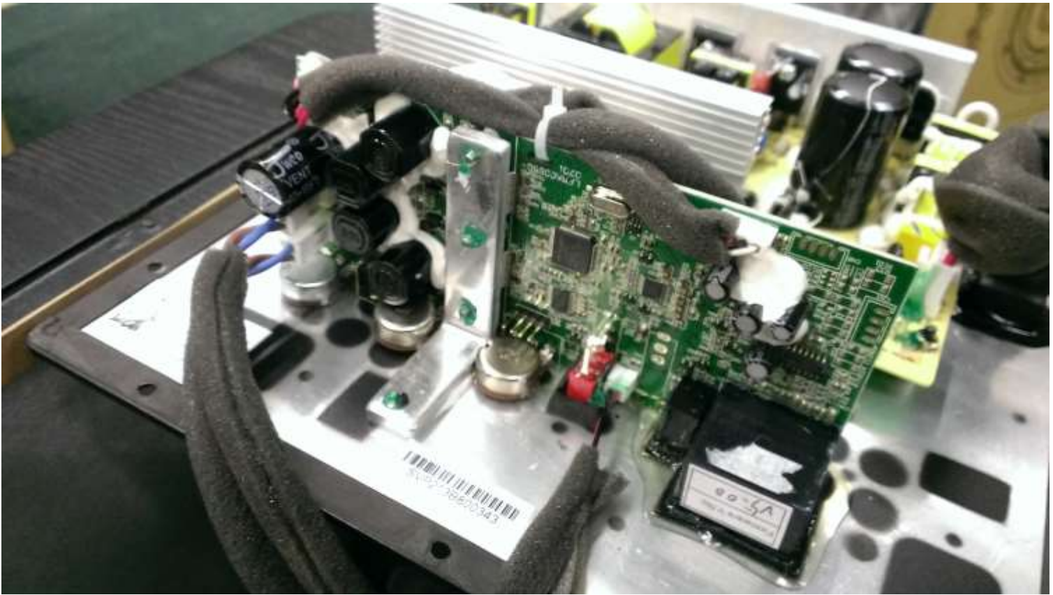
Image #1 –Woofer Lead Wires (larger connectors on left) and LED Lead Wire (smaller connector on right)
