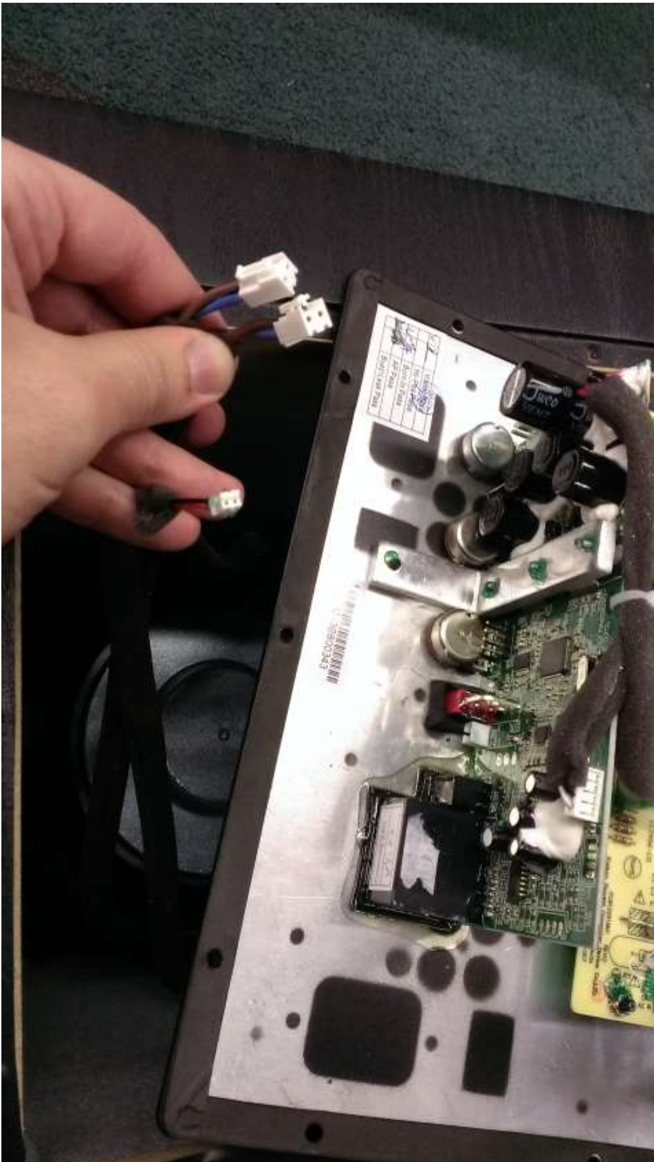
Image #2 – Remove Woofer Lead Wires – Squeeze Release Tab To Remove
