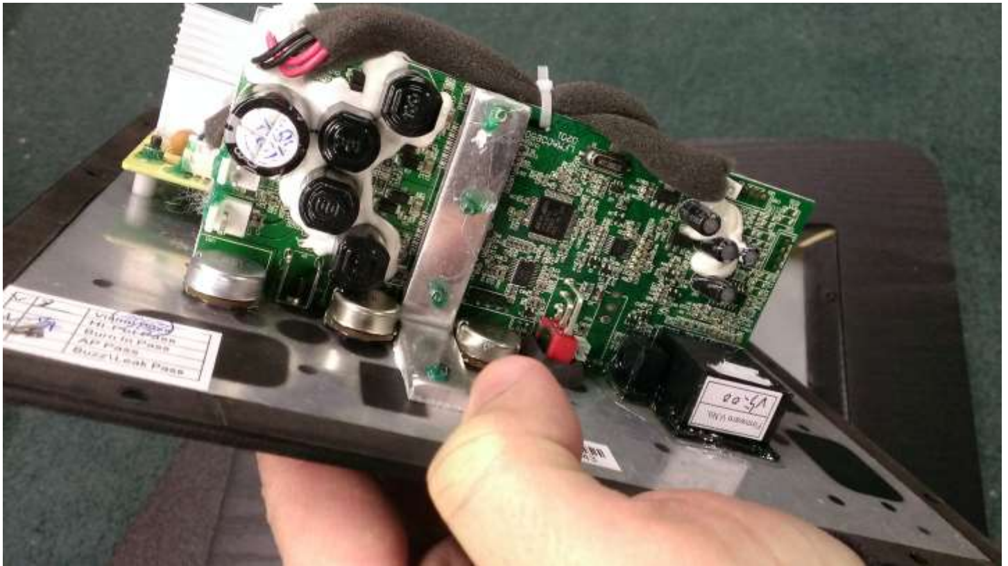
Image #3 – Amplifier Removed From Cabinet With Three (3) Lead Wires Disconnected
