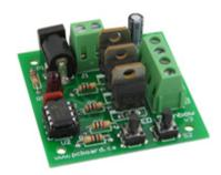
The unique design allows for the selection of various lighting effects and dimming sequences by selecting a routine from the onboard pushbutton. The processor will run pulse width modulation (PWM) to vary the intensity of three outputs (either single LEDs or LED arrays).
