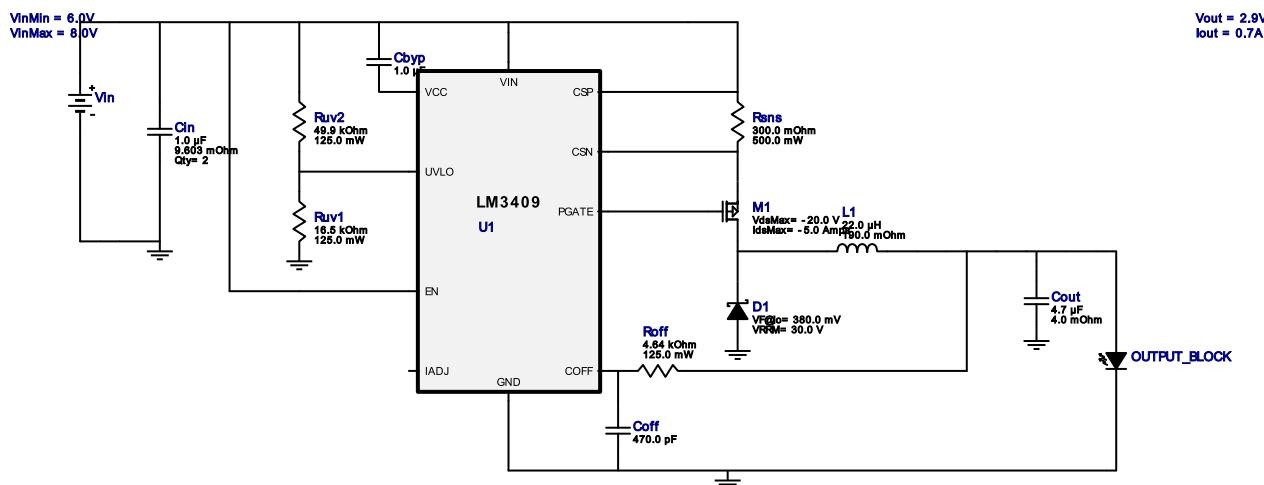
1. Bypass Capacitor Connection : WEBENCH schematic configured for the selected PFET's total gate charge (Qg). If the Qg value is > 30 nC, the Bypass Capacitor(Cbyp or CF) is connected from the VCC pin to CSN pin instead of the typically connected from VCC to Vin when Qg < 30nC.
