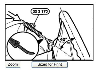
Insert special tool 323170 through bores below an angle of approximately **40°** into steering wheel.
