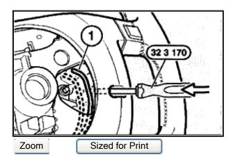
Unlock airbag unit by pressing special tool 323170 in. In so doing, pull airbag unit off steering wheel.
