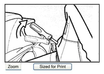
Gently tilt tool in direction of <u>steering wheel</u> until ring spring is engaged in steering wheel (can be felt by a springy resistance).
