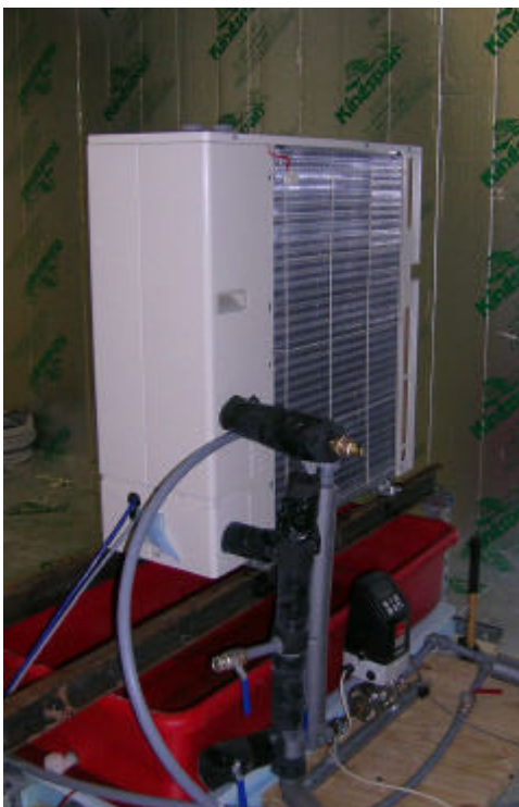
Figure 4 Inlet and outlet temperature sensors and flow meter
