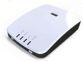
The AP 2MP is a revolutionary MIMO indoor access point designed to bridge the gap between outdoor WISP CPE devices and indoor end-user networking equipment. This provides a vendor-neutral, customer endpoint connectivity solution, all in one device. The AP 2MP provides Power-over-Ethernet to almost any vendor CPE (including Deliberant, Motorola Canopy, Ubiquiti, and Tranzeo) while also providing
