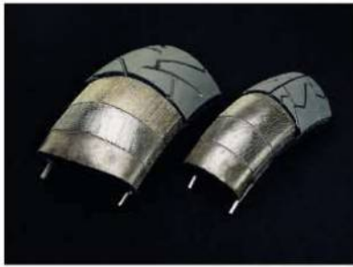
These late-Nineties Bridgestone tyres were among the first to have multi-compound treads, with softer shoulders and a harder centre line
