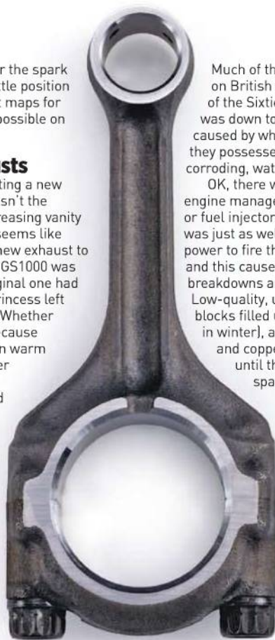
The shape of a modern con-rod is more economical, with fastening studs screwed into the top part, rather than a headed bolt. Better materials, CAD design and improved toughening reduces stresses and improves strength. From this comes higher revs and better reliability
