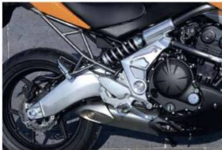
Offset monoshock looks odd but works well
