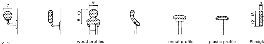
② Handrail profiles
