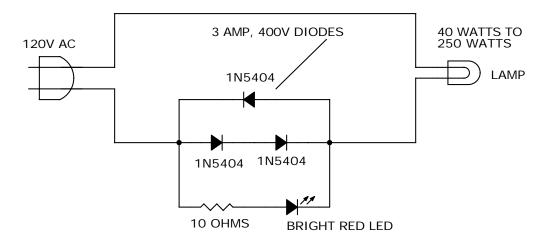
LED LIGHTS WHEN LAMP IS DRAWING CURRENT
