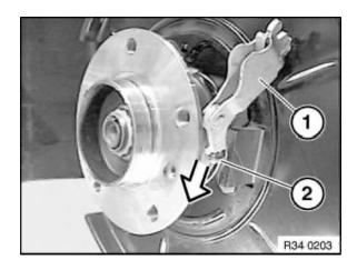
Pull brake shoe expander (1) forwards, disconnect handbrake cable (2) and remove brake shoe expander.
