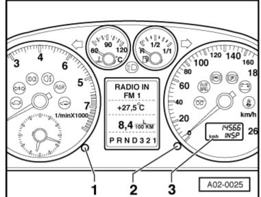
Keep pulling the time setting knob -1- in the dash panel insert until the display is reset.
